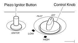
Figure 15 - Control Knob In The OFF Position (Model VN10A Shown)
